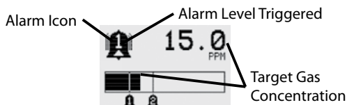
Figure 34. General Status Alarm - detail
