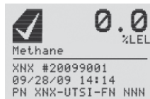
Figure 40. General Status screen with unit information
